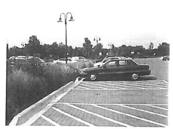
Interlocking concrete pavers work together with curb inlets to provide rainwater to the bioretention area Morton Arboretum, Lisle, IL. Courtesy of Morton Arboretum
