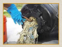
All varieties of wipes will clog sewer lines and damage grinder pumps!
