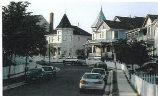
Hamlet residential streets are narrow, allow parking, have sidewalks, and the homes are close to the sidewalk.
